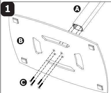
Attach the base to the bottom of the post assembly using the supplied flat head screws (C) and allen wrench (D).
