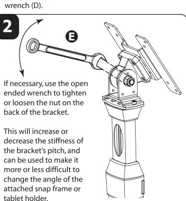
The holes in the bracket at the top of the stand are threaded to accept M5 screws. Use these holes to mount tablet holders or other accessories to the stand. Use the appropriately sized hardware included with those items.
